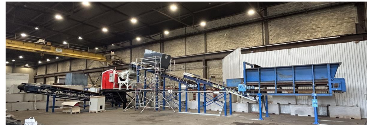
Testline for training and evaluation of sensor systems for shredded scrap
