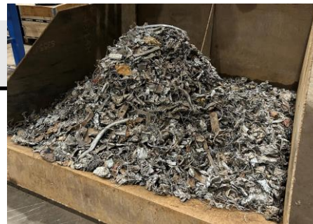
The first batch of complex Fe scrap passed through the system
